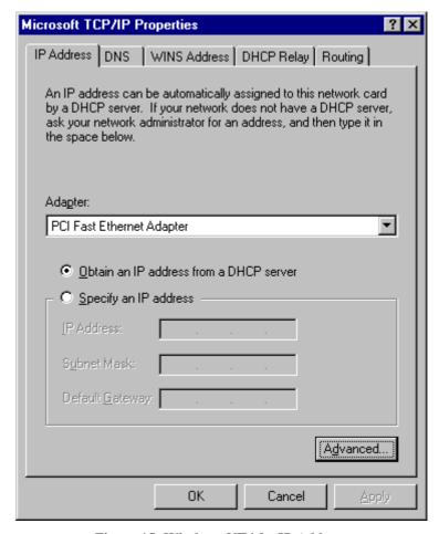
Figure 15: Windows NT4.0 - IP Address
